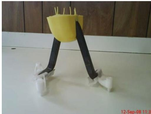
*Figura 3.8 Inserto coil bolt burke*
