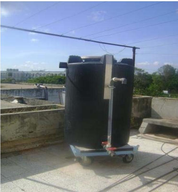
*Figura 2.1 Digestor anaerobio.*
